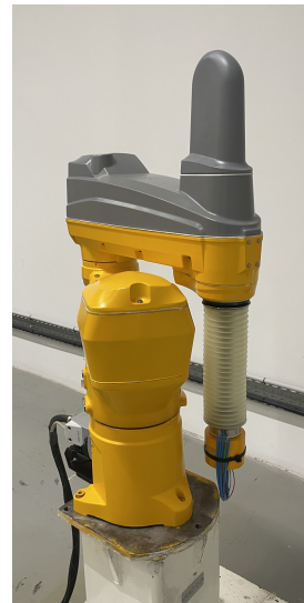
Figure 3: The Staübli 4-links robot manipulator providing the working data used in Section 4. Axis 3 is translational while all the remaining ones are rotational.
